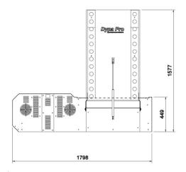
Electrical 190-240V ac Single Phase Max Current 32 Amps Fuse at 32 Amps 6mm<sup>2</sup> Minimum Cable size recommended
